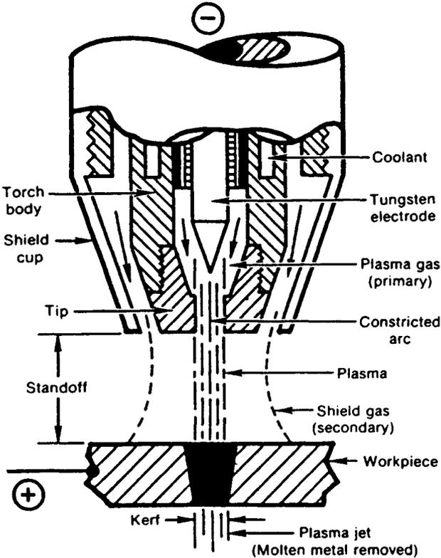
Fig. 33.56 Plasma-beam machining.
