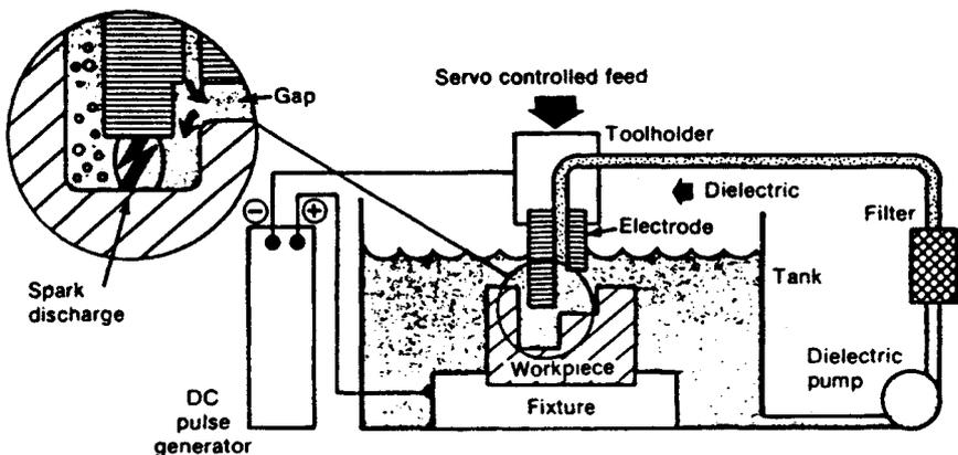
Fig. 33.51 Electrical discharge machining.
