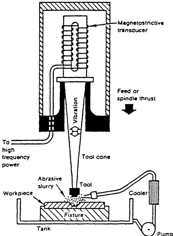
Fig. 33.37 Ultrasonic machining.
