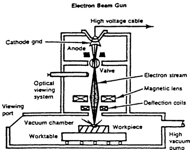
Fig. 33.49 Electron-beam machining.
