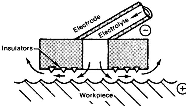
Fig. 33.45 Electrochemical sharpening.
