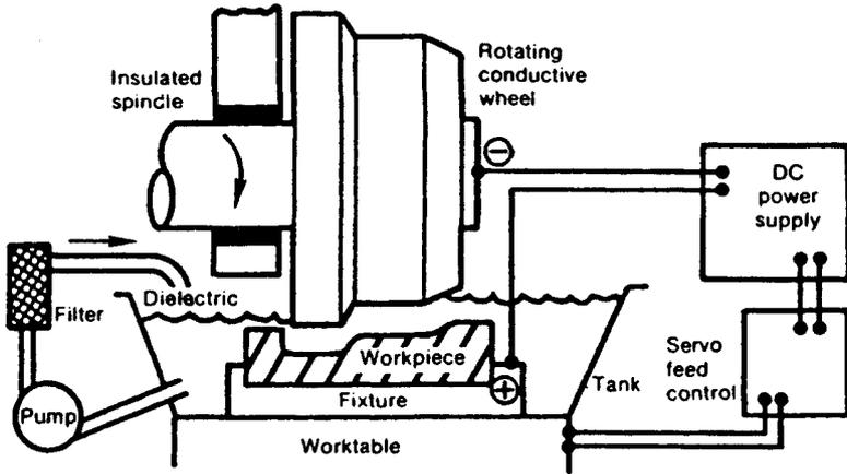
Fig. 33.50 Electrical discharge grinding.
