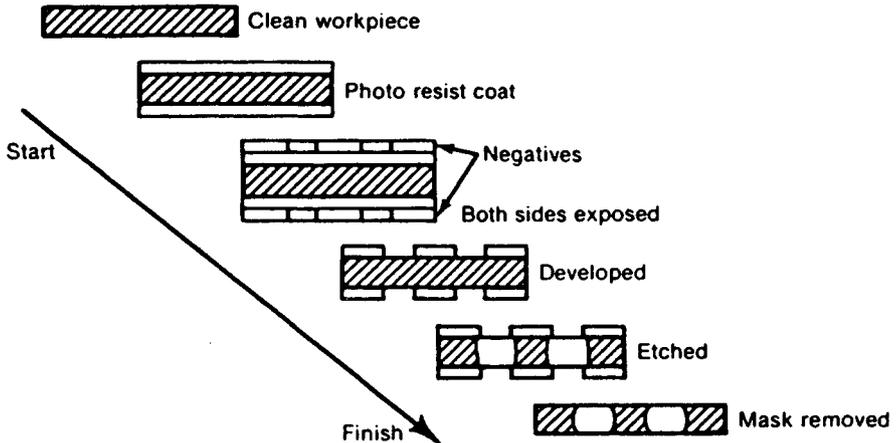
Fig. 33.59 Photochemical machining.
