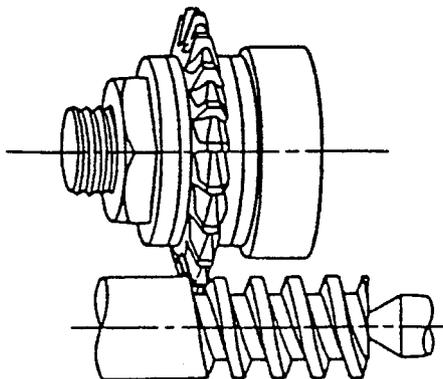
Fig. 33.24 Single-thread milling cutter.
