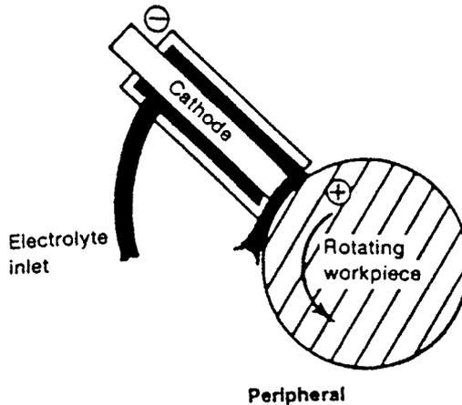
Fig. 33.46 Electrochemical turning.
