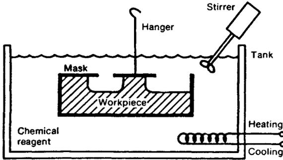
Fig. 33.57 Chemical machining.
