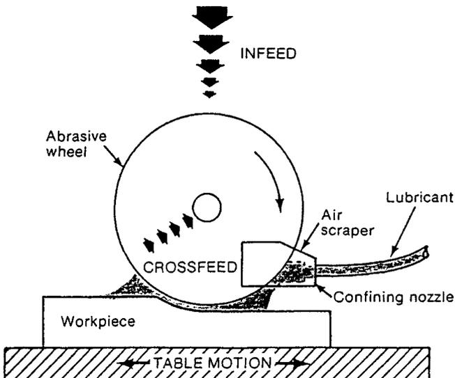
Fig. 33.34 Low-stress grinding.
