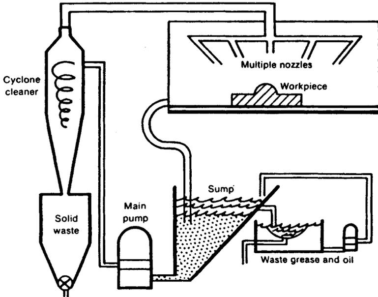
Fig. 33.38 Water-jet machining.
