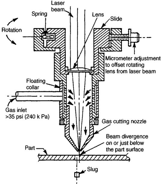
Fig. 33.55 Laser-beam torch.
