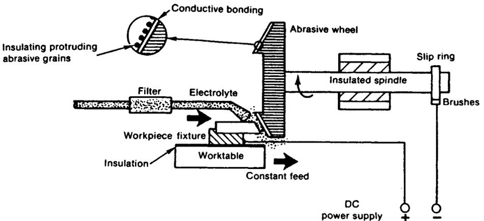
Fig. 33.41 Electrochemical grinding.
