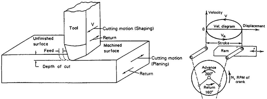
Fig. 33.28 Basic relationships of tool motion, feed, and depth of cut in shaping and planing.
