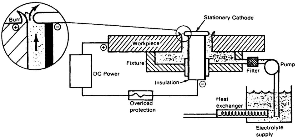
Fig. 33.39 Electrochemical deburring.
