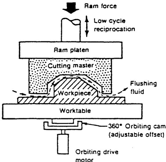
Fig. 33.36 Total form machining.
