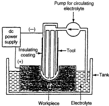
Fig. 33.43 Electrochemical machining.
