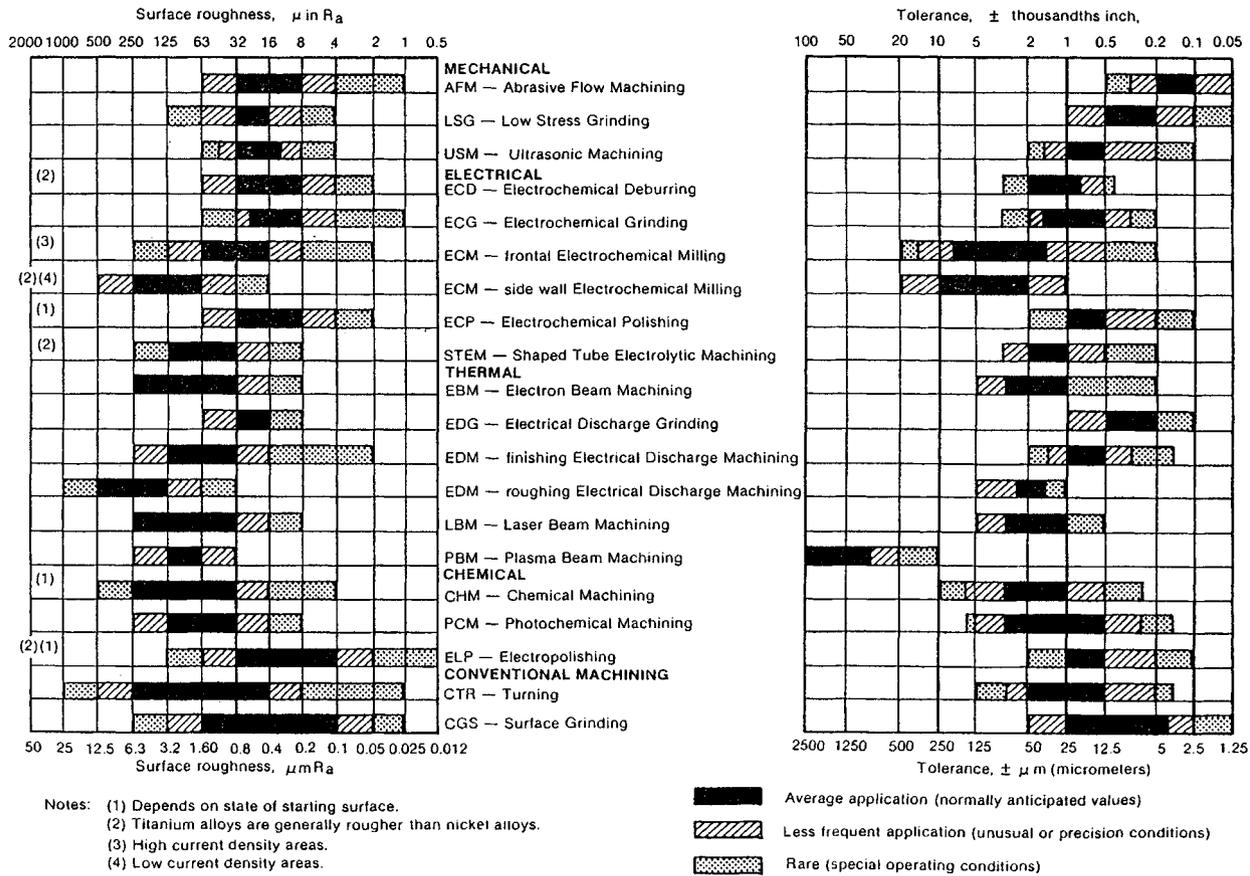
**Fig. 33.30** Typical surface roughness and tolerances produced by nontraditional machining.
