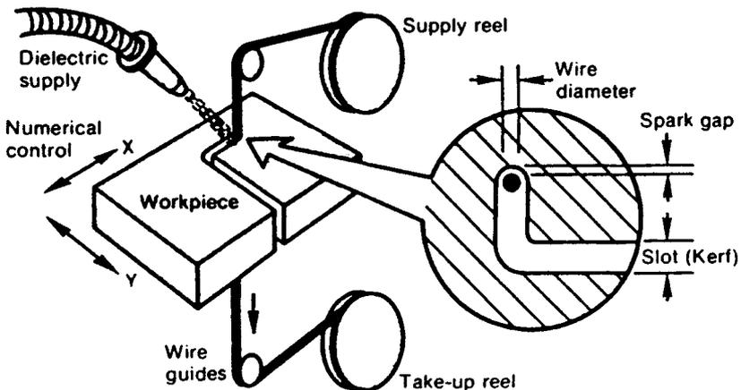
Fig. 33.53 Electrical discharge wire cutting.
