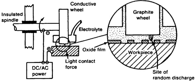
Fig. 33.40 Electrochemical discharge grinding.
