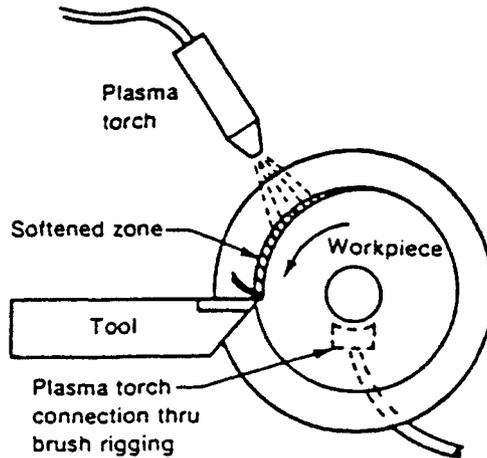
Fig. 33.35 Thermally assisted machining.
