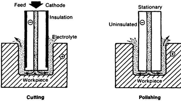
Fig. 33.44 Electrochemical polishing.
