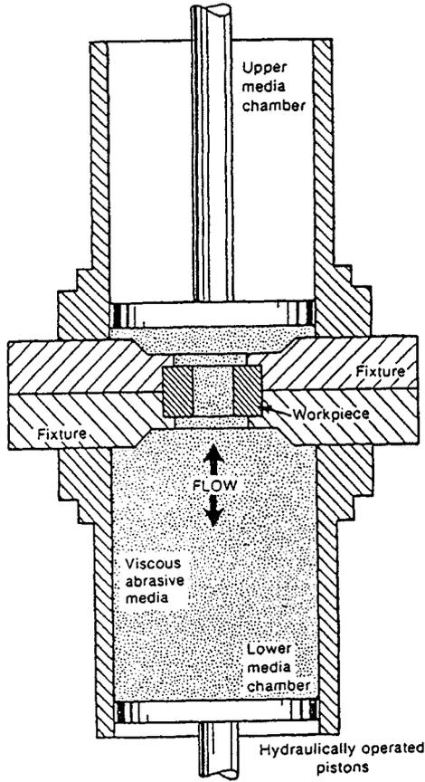
Fig. 33.31 Abrasive flow machining.
