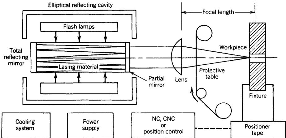
Fig. 33.54 Laser-beam machining.
