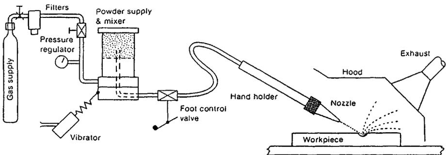
Fig. 33.32 Abrasive jet machining.
