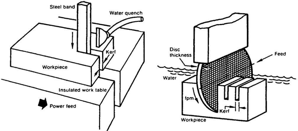
Fig. 33.52 Electrical discharge sawing.
