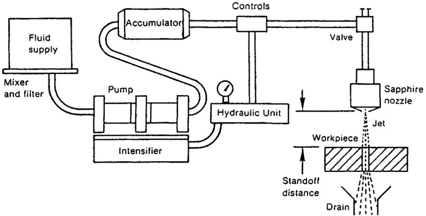
Fig. 33.33 Hydrodynamic machining.
