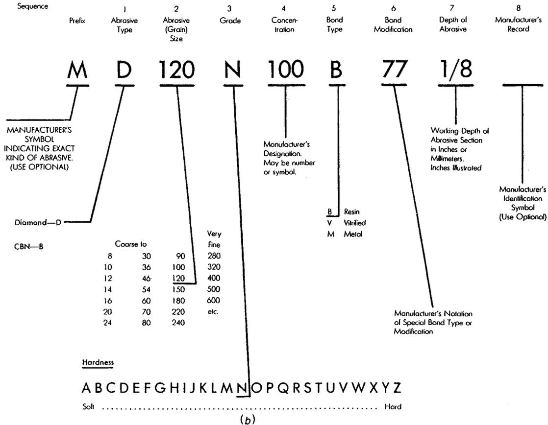
**Fig. 33.29** Standard systems for grinding wheels. (a) aluminum oxide, silicon carbide; (b) diamond, CBN.
